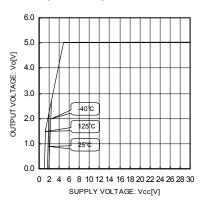
Fig.2 Line Regulation (Io=0mA)
