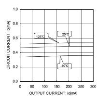
Fig.8 Circuit Current (lo=0mA→300 mA)
