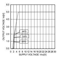
Fig.3 Line Regulation (Io=200mA)
